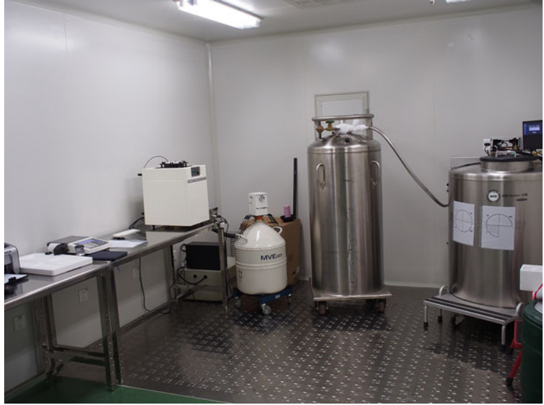
Fig. 4 Separate ovarian tissue freezing room within the clean room area. The freezing device is located on the left side and connected to a nitrogen supply tank. The cryotank for long-term storage ( right side ) is connected to a separate nitrogen supply tank located in the middle
