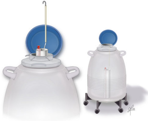
Fig. 6 Short-term storage of semen samples in liquid nitrogen tanks. Reprinted with permission, Cleveland Clinic Center for Medical Art & Photography © 2010–2013. All Rights Reserved
