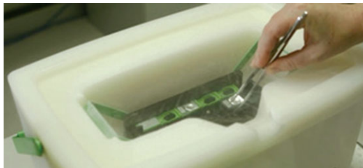
Fig. 11 Working station. Place cassette on internal metal block using the magnets to locate and secure the cassette in place
