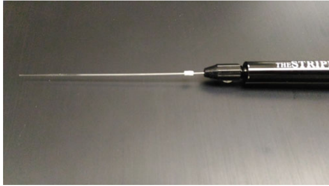
Fig. 8 A stripper (capacity 275 \mu\text{L} ) with silicon seal connected to handle used to pipette less than 3 \mu\text{L} sperm suspension with sucrose buffer
