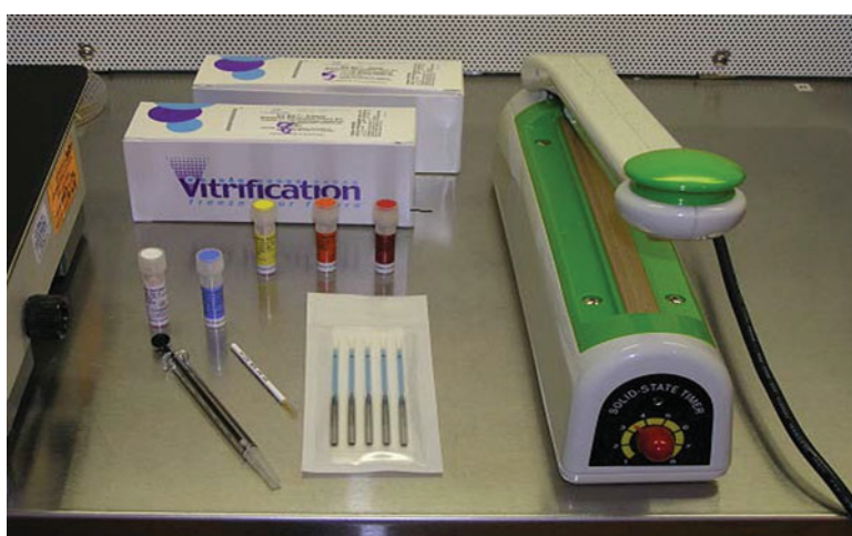
Fig. 5 Materials required at workstation: Vit Kit®, CryoTip®, labeled straws, impulse heat sealer, 25 µL Hamilton Gastight Luer Tip Syringe, and connector
