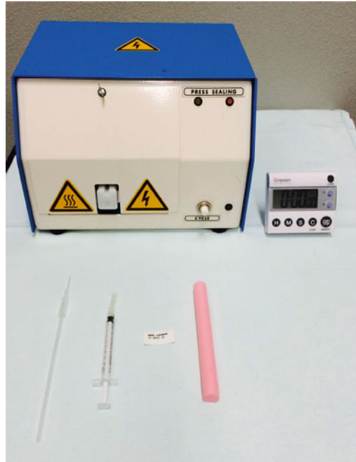
Fig. 1 Equipment necessary for slow freezing. From the left in the upper of the image: impulse-heatsealer, timer. From the left in the lower of the image: sterile straws, insulin type syringe 1 ml connected to a silicone tube, label (name, surname, sample number, date, couple code) and goblet
