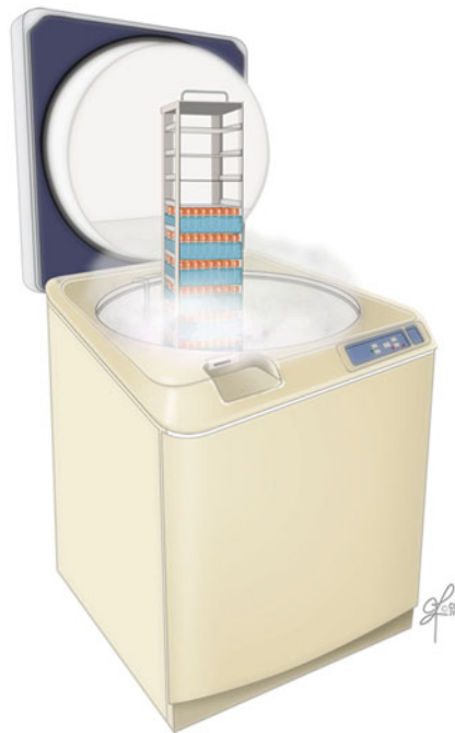
Fig. 7 Long-term storage of semen sample in liquid nitrogen tank. The figure shows a metal canister containing boxes filled with cryovials. Reprinted with permission, Cleveland Clinic Center for Medical Art & Photography © 2010–2013. All Rights Reserved
